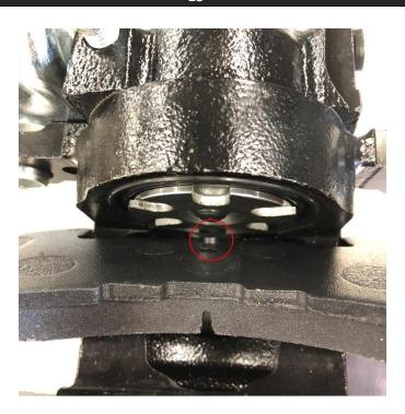
**Kits with parking brake calipers** do not use a machined pad spacer and should be checked to confirm the pad is seated flat against the piston face, with the boss of the brake pad lining up with the notch in the piston face.
